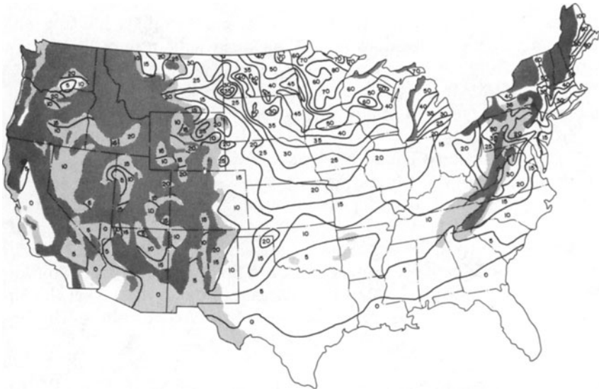
Fig. 6.3. Fifty-year recurrence interval ground snow map in pounds per square foot ( S_g ). Dark shaded areas are where the variation precludes mapping at this scale. Lighter shaded areas are where available data should be applied with caution. (Load is in \text{kg/m}^2 = 4.88 \text{ lb}_m/\text{ft}^2 .) From ANSI Standard A58.1-1982.
